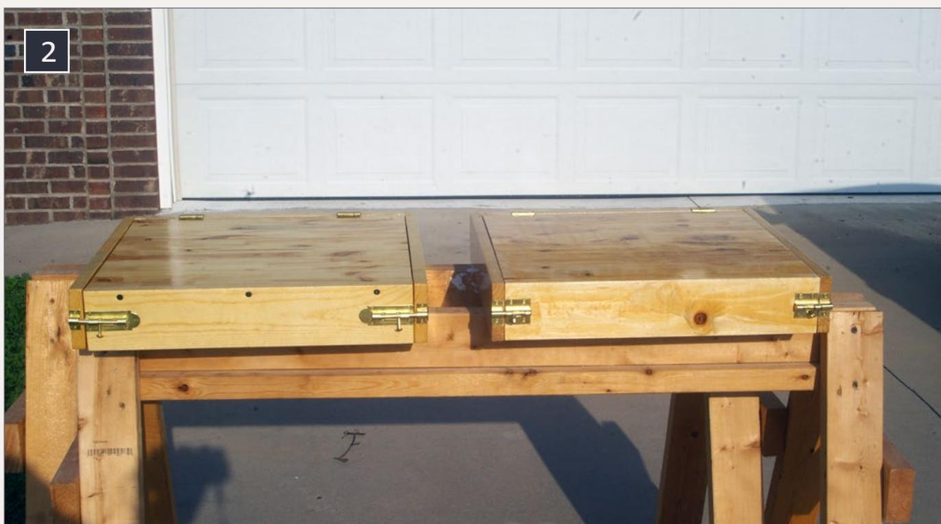
**2. This is the workbench when closed. It's simply a box, 17½" deep, 19½" wide, and 3½" tall. The barrel bolts keep it closed, and also prevent the lid from closing too far and potentially crushing the contents. Attaching the box front to the lid leaves a convenient opening so you're not working down inside the box, while still having the other three sides to keep tools and parts from falling off.**
