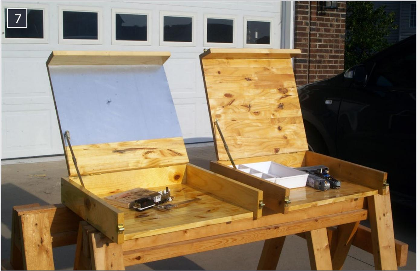
7. There are a few differences between the two workbenches. The second one (left) has a small lip to prevent anything from rolling out. Rather than cutting a groove in the bottom board, you could use edging veneer designed for hiding the edges of plywood, or even heavy cardstock. Once glued in place and varnished, it would be more than strong enough.
