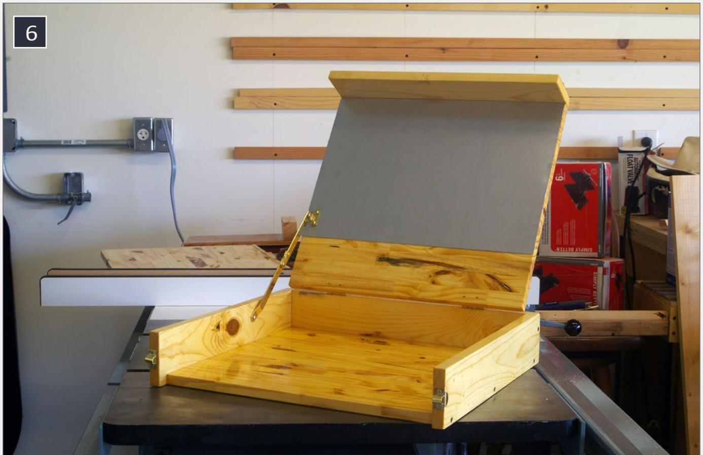
**6. For the first workbench, I mounted the folding support bracket  $5\frac{1}{2}$ " forward from the back edge of the top. Although it works, the top opens just far enough to make me worry the workbench could tip over backward. For the second one, I mounted the bracket  $\frac{1}{4}$ " farther forward, and you can see the resulting change in the angle.**
