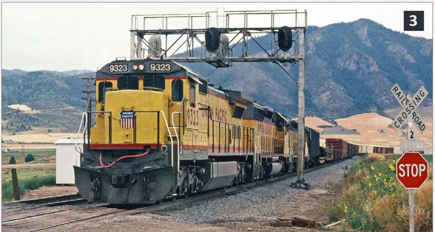
**3. A Union Pacific freight rolls under a signal bridge on the nine-mile stretch of two main tracks at Blaser, ID in 1990. The bridge carries signals for traffic in both directions on both tracks. Josef Brugger photo.**
