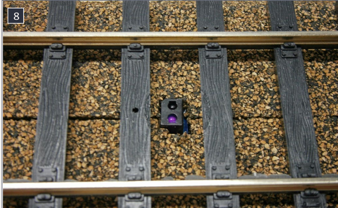
8. The sensor mounted below the track.
