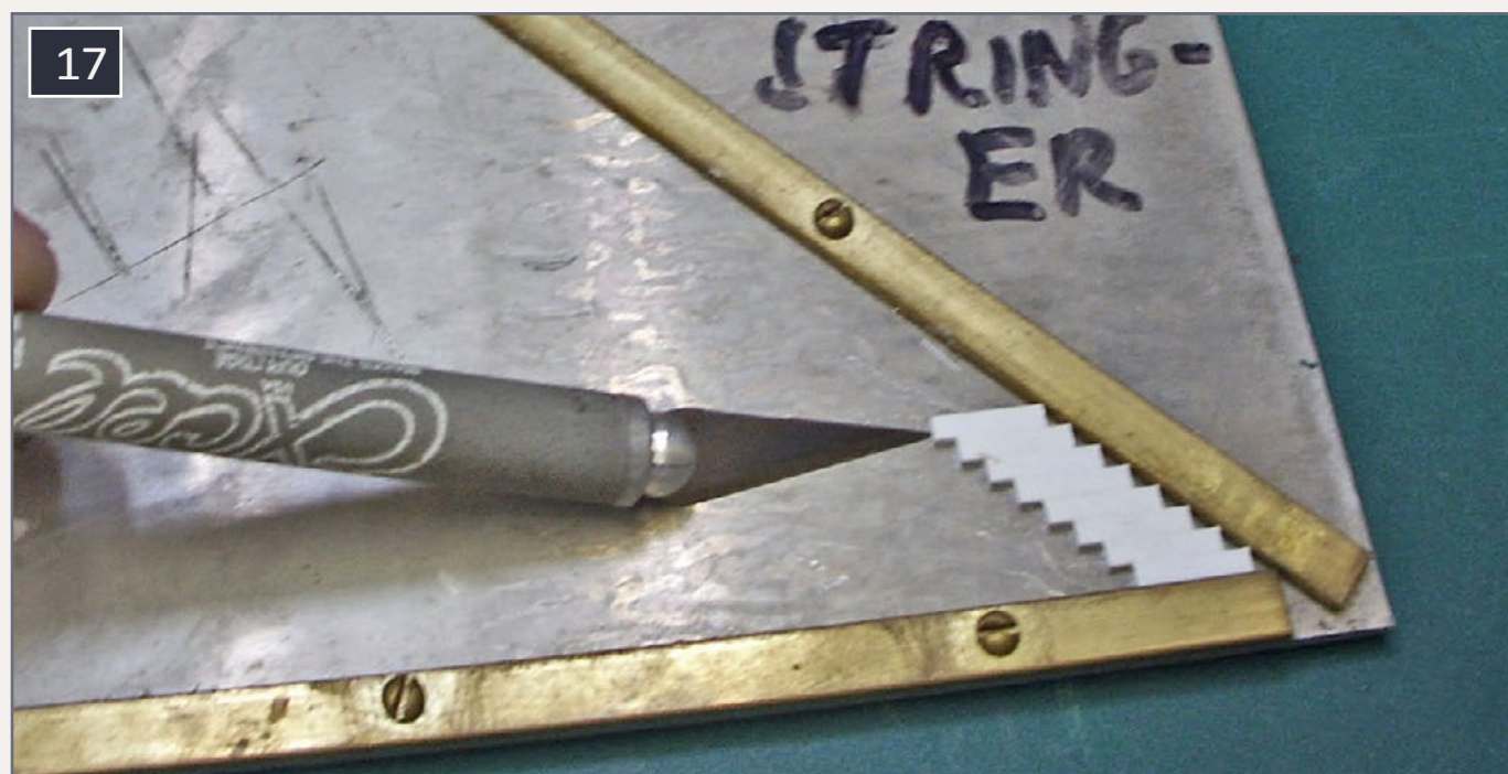
17. 4 x 8's are stacked against the edge of the jig until I have the desired height for the stairs.
