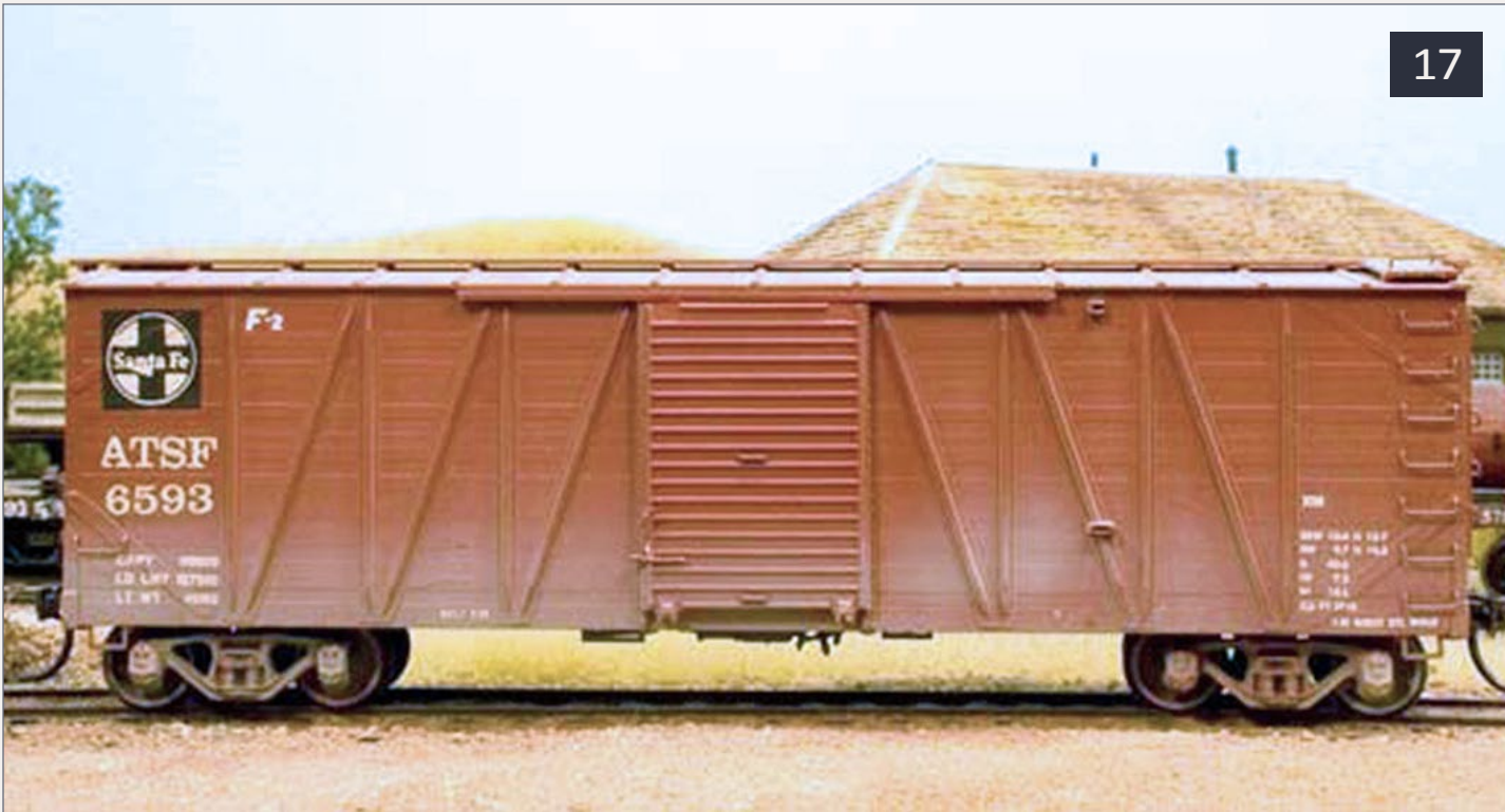
17: This boxcar has a typical weathering job applied with an airbrush using solvent-based paints. Light mud and gray were sprayed on the bottom edge of the body and on the trucks. Using an airbrush offers precise control over the amount of paint on the model, and makes it easy to apply a very light mist of paint that mimics dust and dirt blown up from the roadbed. Car modeling and weathering by Dick Truesdale.
