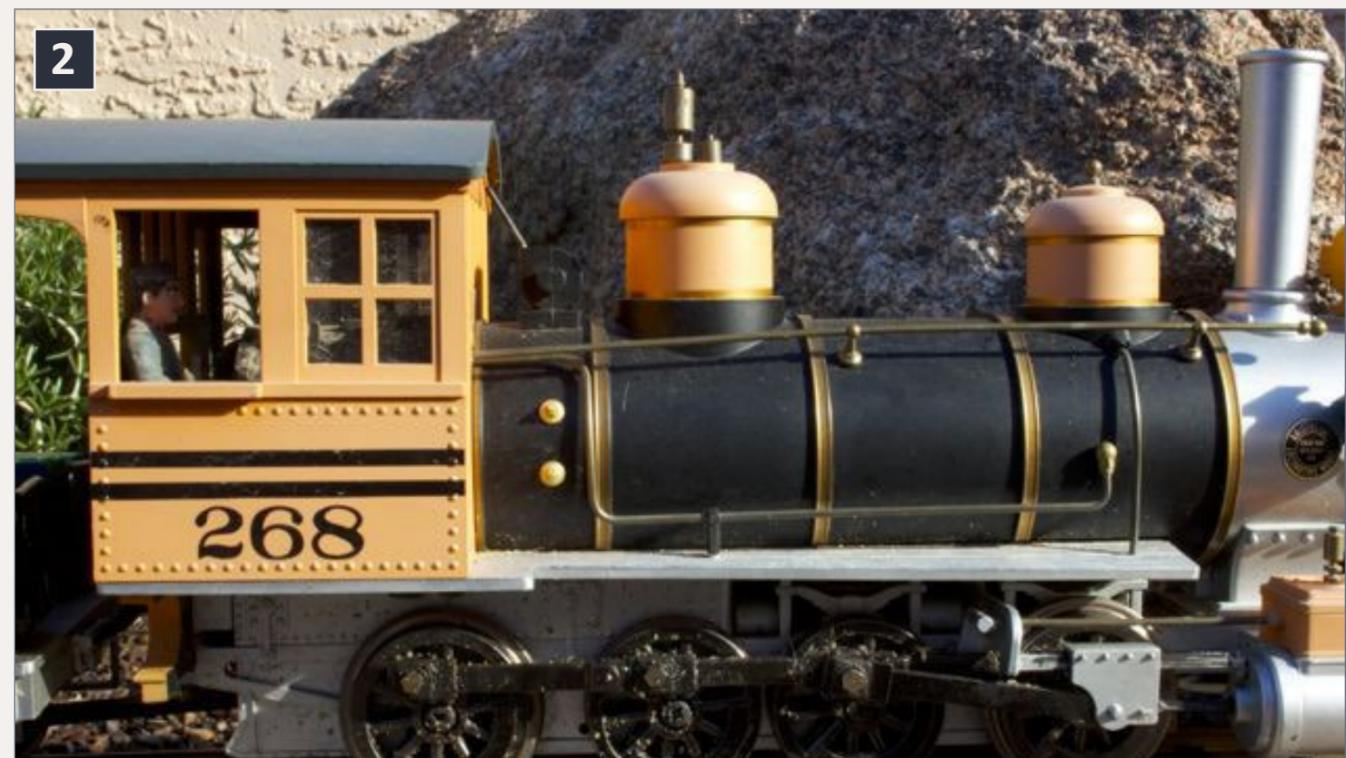
**2: Loco with cab address of 268 – this will be a long address on any system, even though it has only 3 digits.**
