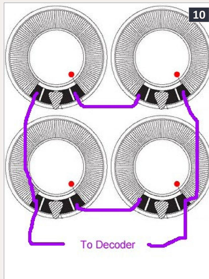
**10: Four speakers in a series-parallel array – the final impedance will be the same as the speaker impedance – 8-ohm speakers will yield an 8-ohm load.**
