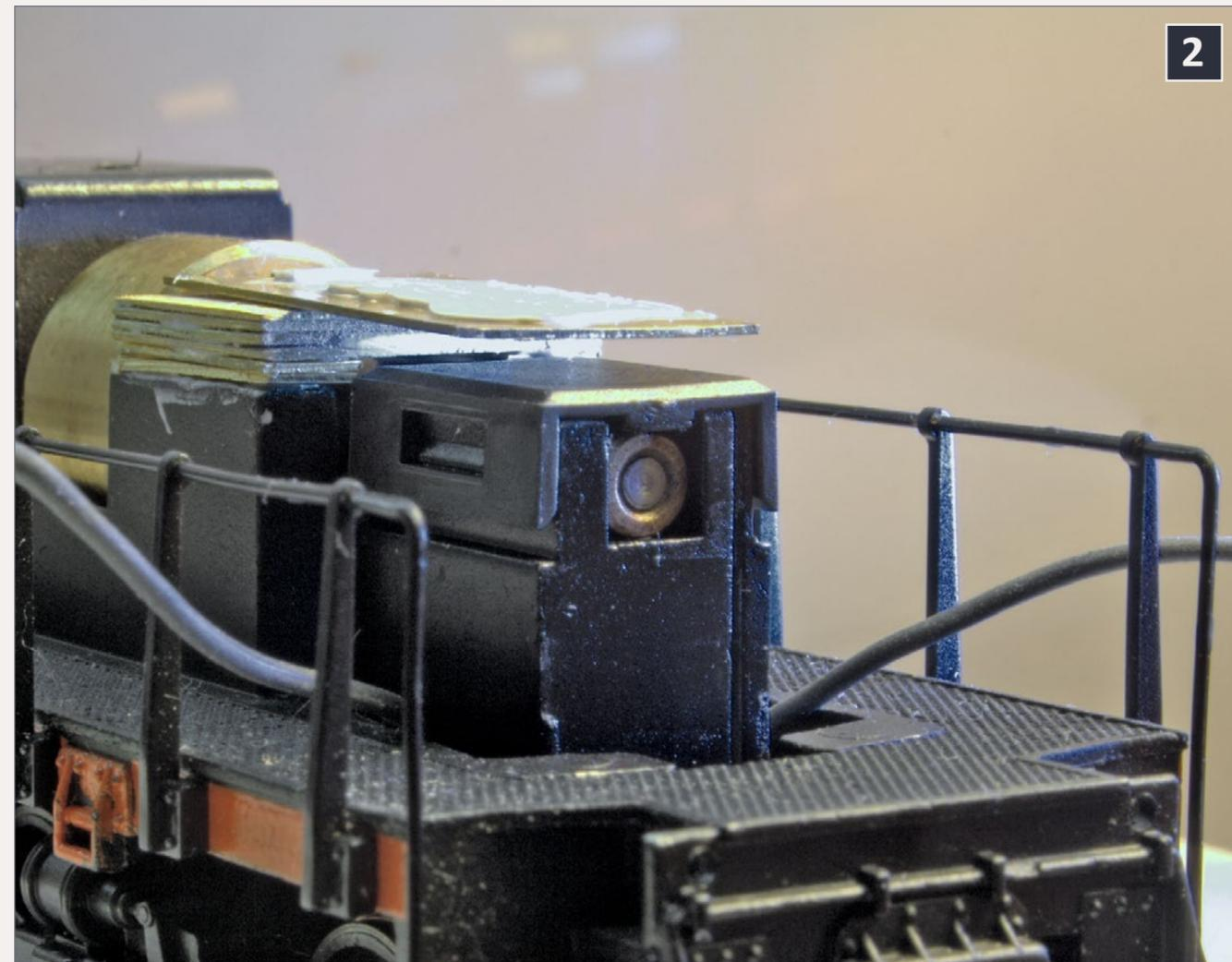
**2: Atlas HO scale S-2 loco with brass riser and plate for mounting a TSU-750 Micro Tsunami decoder. The brass conducts the heat from the decoder into the frame of the loco and is glued together with thermally conductive epoxy.**
