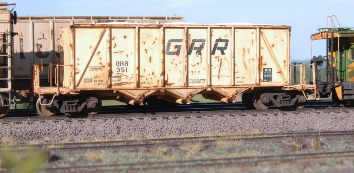
5: This Walthers Ortner rapid-discharge hopper has factory paint. The car is upgraded using brass wire, angle and flat bar for all of the handrails and stirrup steps. The underframe is detailed with brass angle, and Kadee springs for the actuators. Sergent couplers are added. The model was weathered with oils and pastel chalks.
