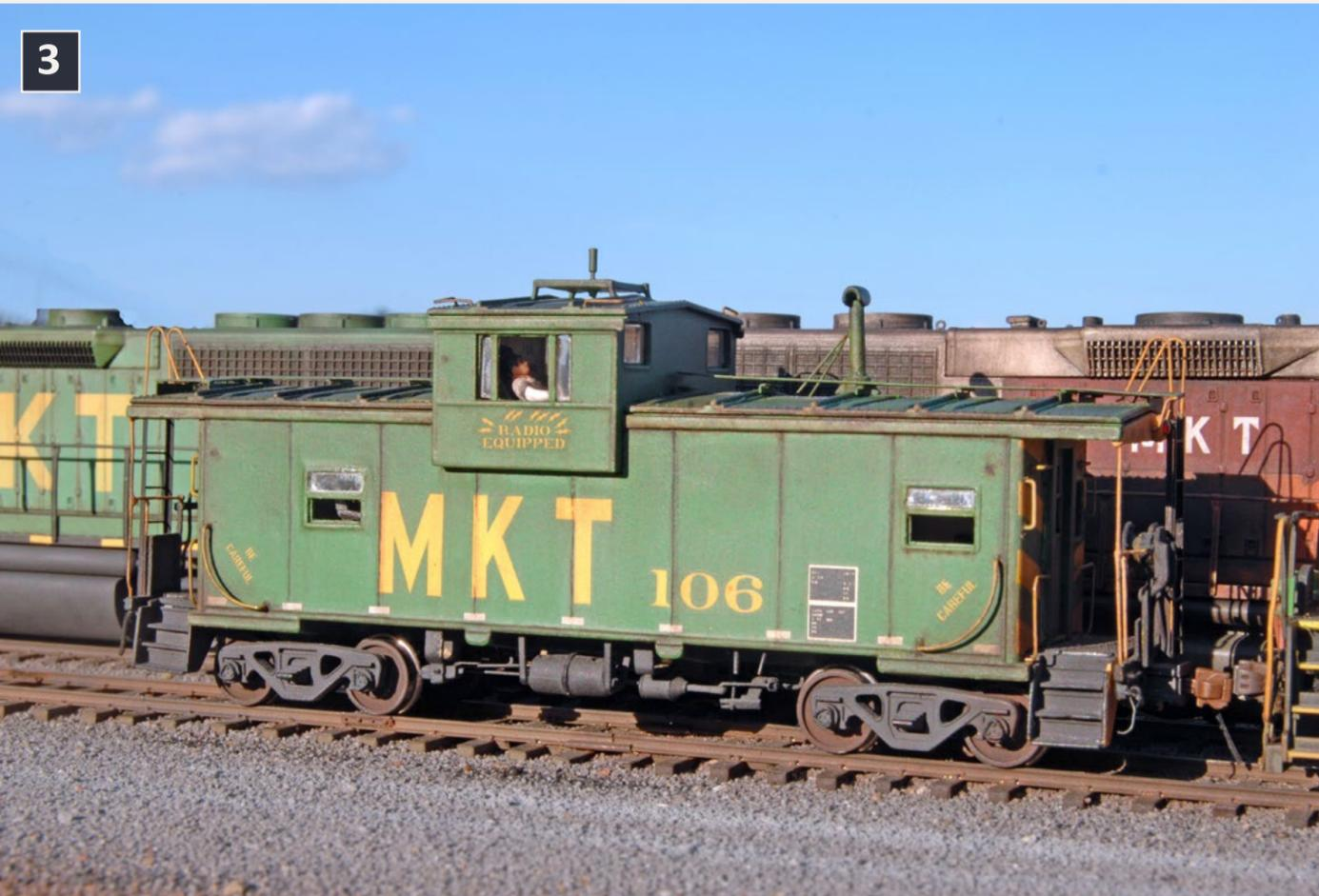
3: On an Atlas cabooses, Scott relocated the side windows, raised the cupola, rebuilt the end cages, and blanked one window on each end. He also detailed the interior and built a full underframe. The paint is Modelflex MKT Green, with Microscale decals. All weathering is by hand, with oils and pastel powders.
