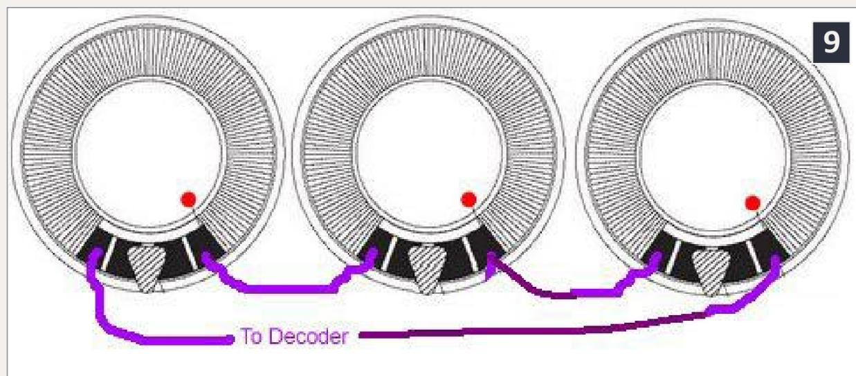
**9: Three speakers wired in series – the final impedance will be three times the speaker rating – 4-ohm speakers yield a 12-ohm load.**
