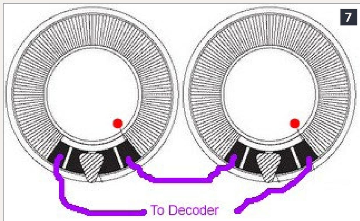
**7: Two speakers wired in series – the final impedance will be twice the speaker rating – 8-ohm speakers yield a 16-ohm load or 4-ohm speakers yield an 8-ohm load.**
