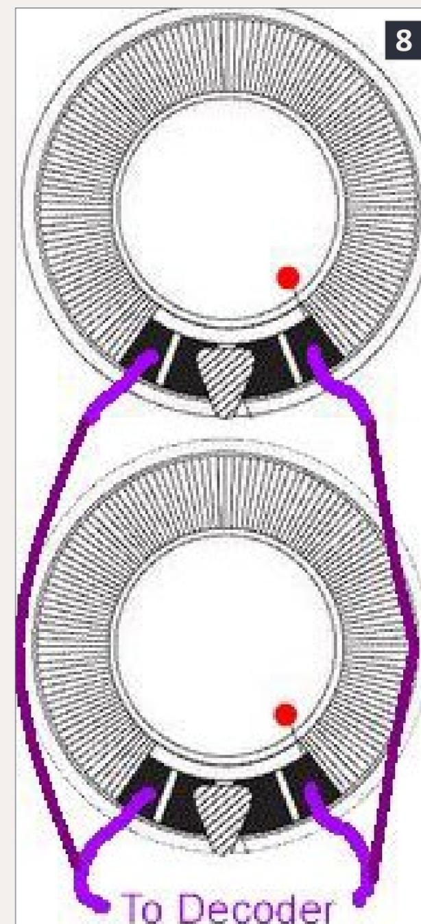
**8: Two speakers wired in parallel – the final impedance will be half the speaker rating – 8-ohm speakers yield a 4-ohm load.**
