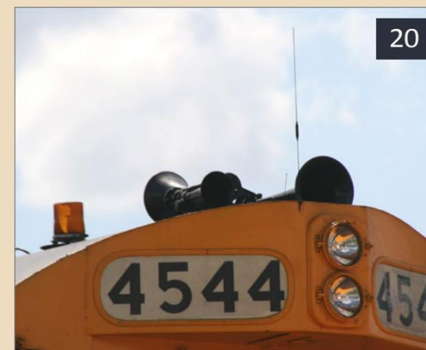
**19-20: The roofs of this maintenance truck and a locomotive show two installations of whip antennas. Whips are generally mounted near the center of a roof to create a ground plane which optimizes the performance of the antenna.**
