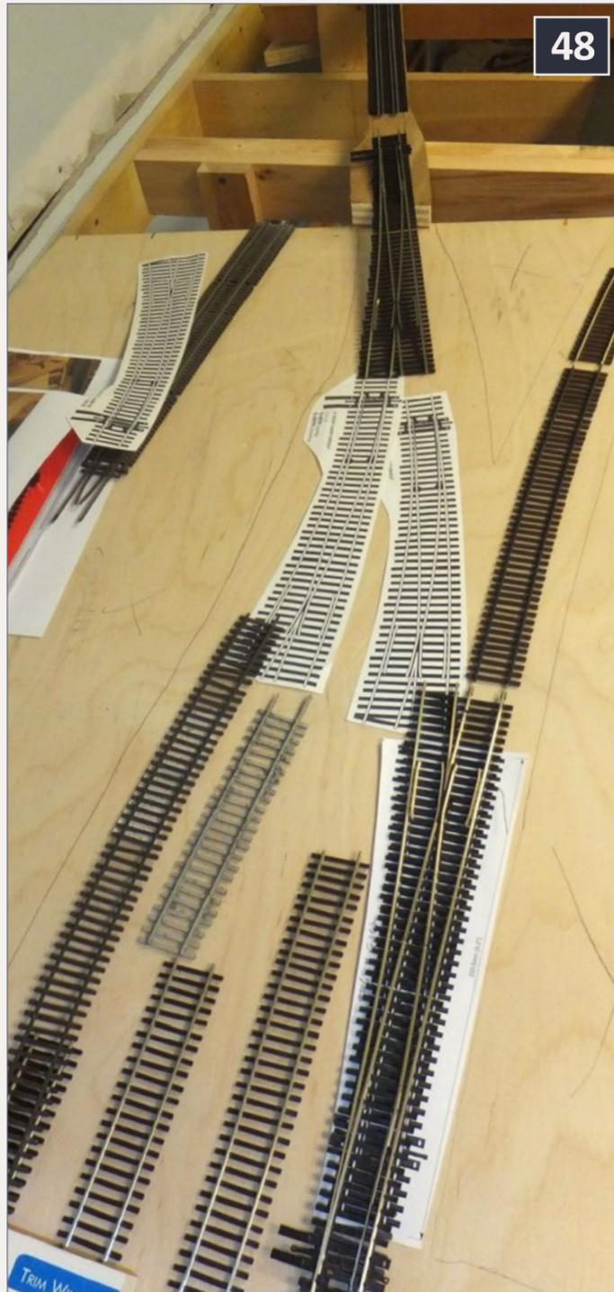
48: Peco makes some very handy turnout templates that are a free download from their website. I planned to use a mix of code 70 and code 83 track and turnouts in this area, since I really needed a few of Peco's curved #8 turnouts. Yet I was connecting with an area that was all done with code 70 track and Micro Engineering turnouts.
