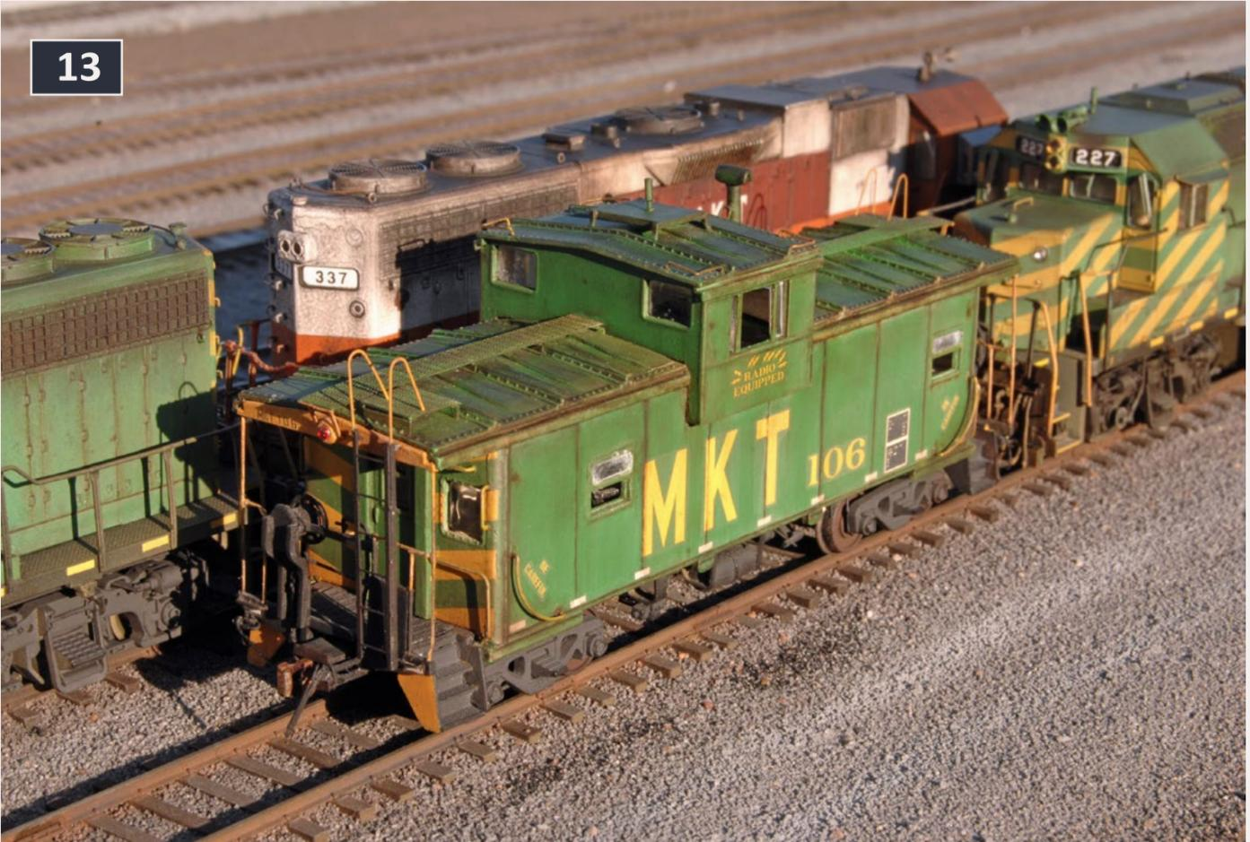
13: Scott reworked the windows, cupola, end cages, and underframe on this MKT caboose. The interior and underframe are fully detailed. Modelflex MKT Green and Microscale decals finished it up.
