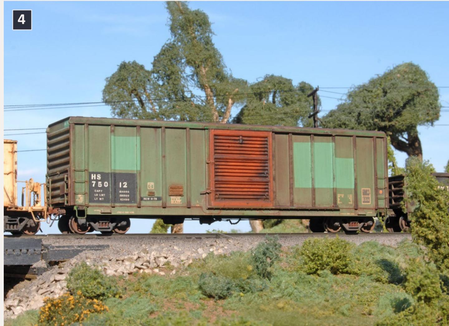
4: The Athearn PS 5344 boxcar is a factory-painted Texas & Mexican, with new data and patches added using Microscale thin trim film. Complete details are added to the underframe. The car has Sergent couplers and is weathered using oils and pastel powders.
